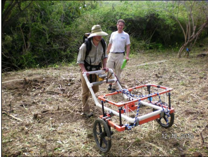
Photograph 61: DGM equipment in DPO
