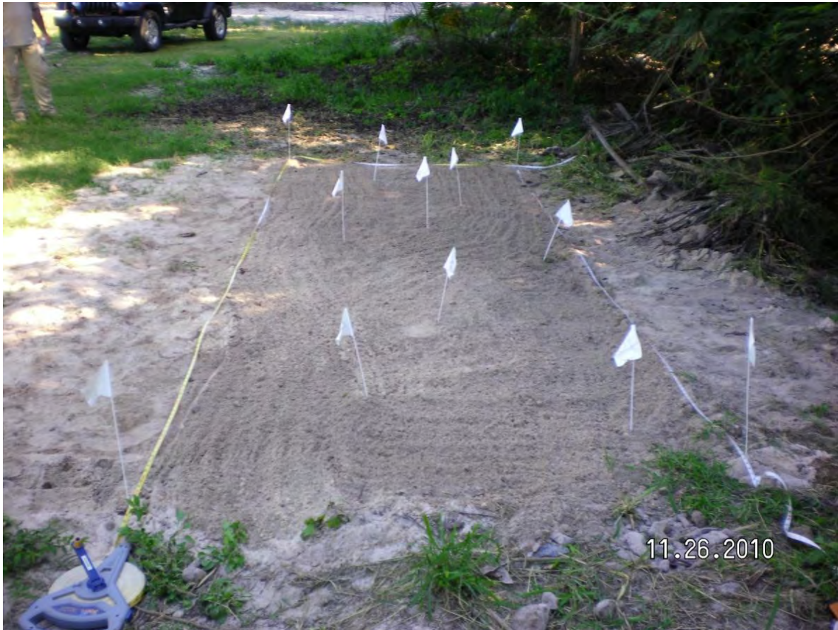
Figure 16 – Geophysical Test Strip used to Evaluate Analog instruments
